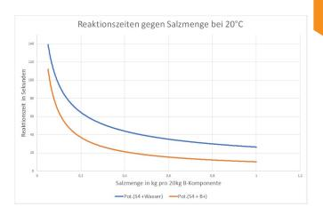
As with all reactions with injection gels, the reaction time is always dependent on the material temperature. The following diagram may be used for approximate orientation, measured for the standard mixture without KÖSTER B +:
